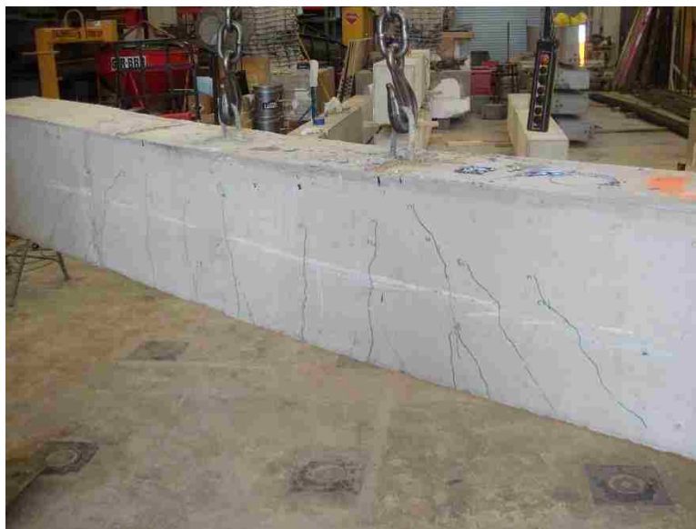
Figure 4.34. Failure of Beam 2
