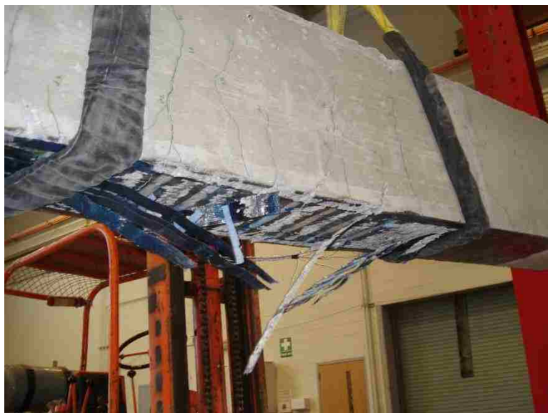
Figure 4.61. Failure of Beam 9
