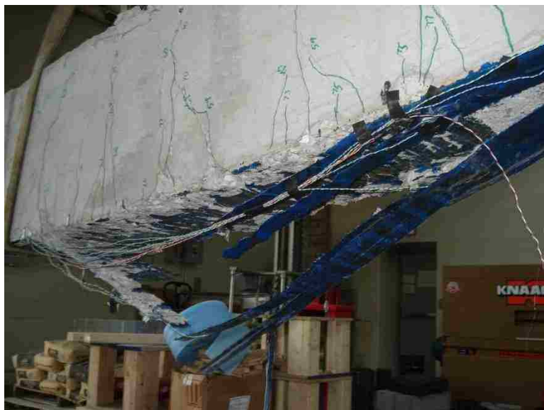
Figure 4.18. Failure of Beam 3
