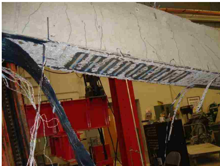
Figure 4.56. Failure of Beam 7
