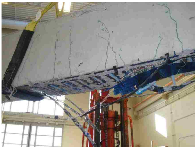
Figure 4.51. Failure of Beam 6
