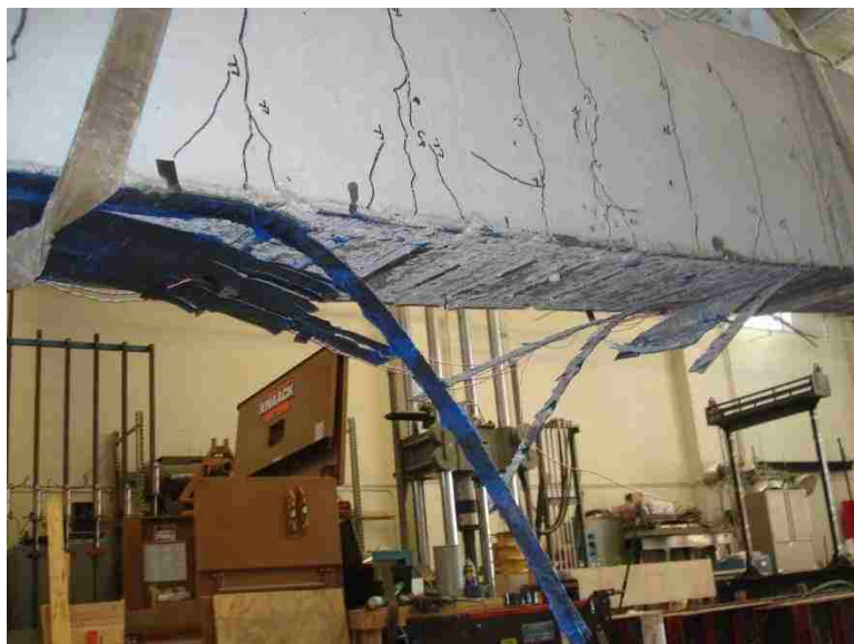
Figure 4.41. Failure of Beam 4
